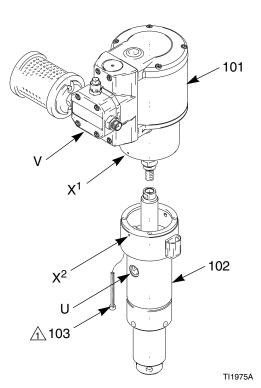
Fig. 4. Pump Connection
