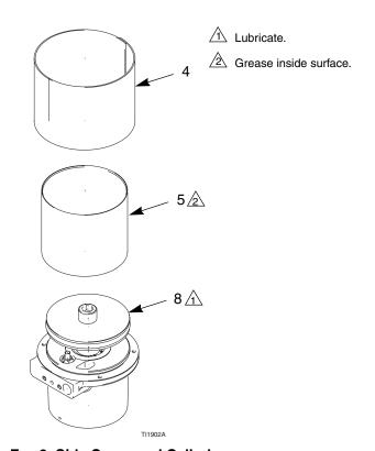
Fig. 9. Side Cover and Cylinder
