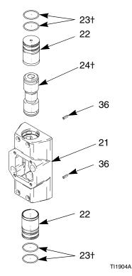
Fig. 7. Air Valve Piston Assembly
