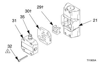
Fig. 6. Air Valve Cover, Seat, and Cup
