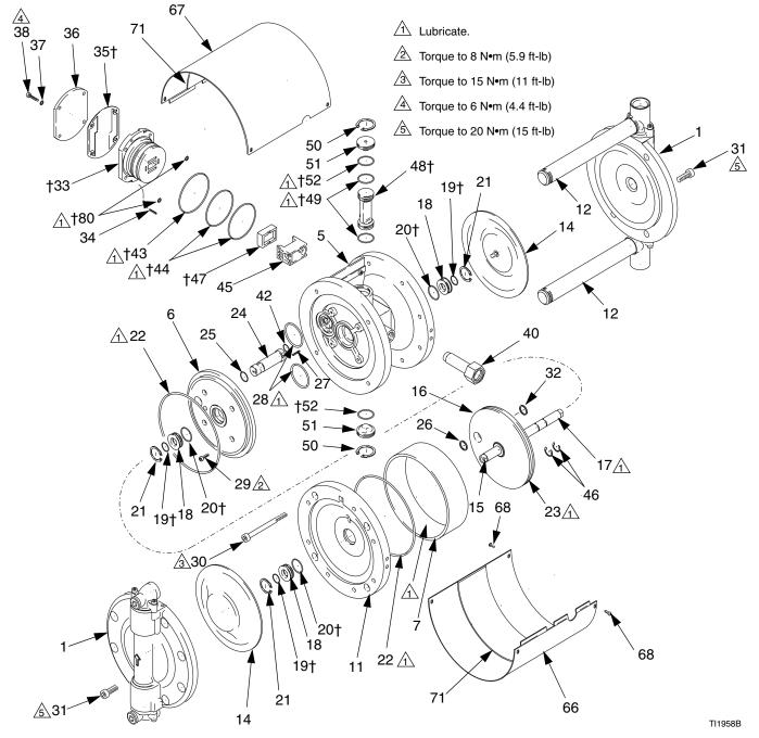
FIG. 7. Repair the Air Valve
