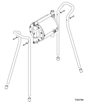
FIG. 2: Floor Stand Installation
