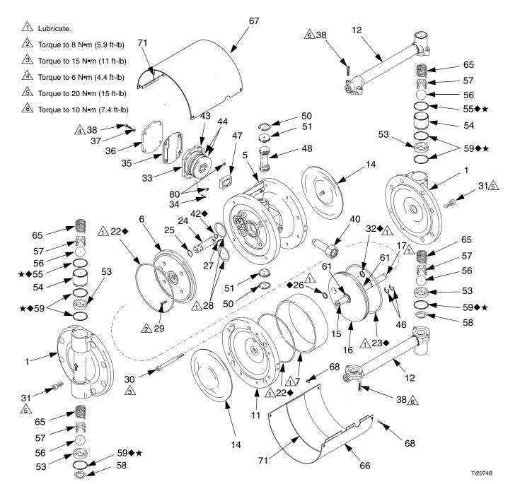
FIG. 9. Replace the Cylinder and Piston Seals
