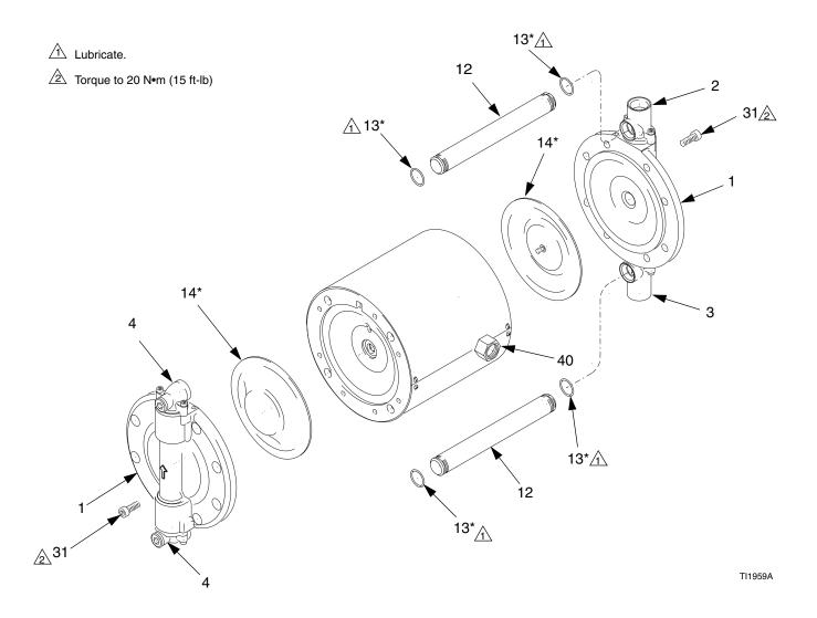
FIG. 6. Replace the Diaphragms
