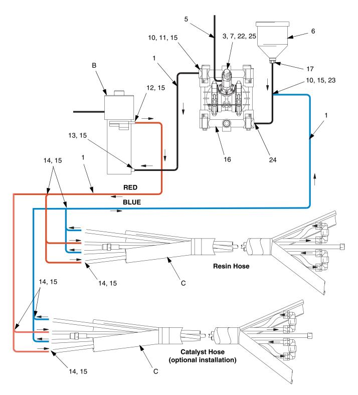
Fig. 1: Fluid and Air Line Connection Schematic
