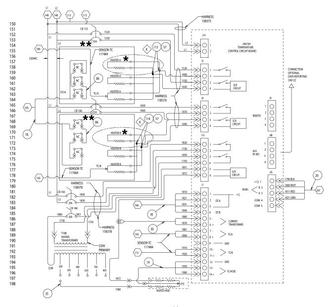
\* Only E-XP2 and E-30, with 15.3KW of heat, Models use 3 heaters per side.
