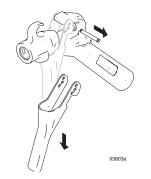
10. Unscrew packing nut (5) from gun body (17).
