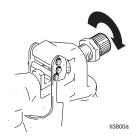
7. Carefully unscrew and remove spring retainer (15) and spring (13) from gun body (17).
