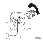
7. Unthread spring retainer (16) and remove spring (14).
