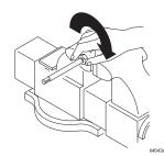
3. Insert needle (8) into packing nut (5).
