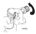
20. Install o-ring (10) on adapter (9).
