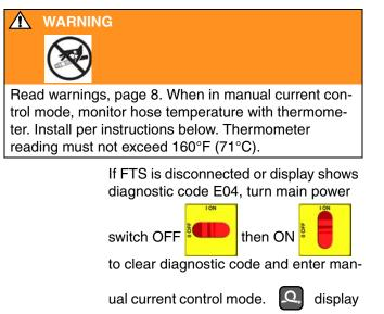
will show current to hose. Current is not limited by target temperature.
