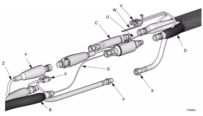
FIG. 5. Install Fluid Temperature Sensor (FTS)
