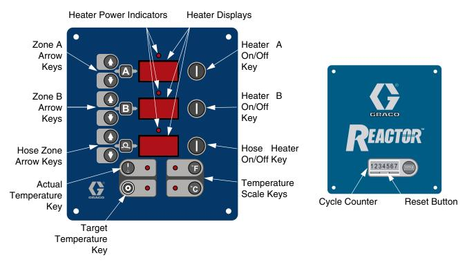
FIG. 4. Controls and Indicators
