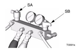
After changing drums, set PRESSURE RELIEF/SPRAY valves to PRESSURE RELIEF. This provides sufficient fluid velocity to purge air from pumps and heaters.
