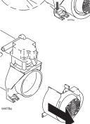
3 Remove fan bolt from center of fan and remove fan from housing.
