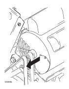
2 Remove ground nut and disconnect green ground wire.
