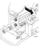
7 Slide feet on the bottom of hose bracket, into the slot on the bottom of sprayer.
