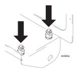
2 Slide new motor into sprayer frame, aligning motor frame opening under bolts. Tighten bolts.
