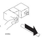
2 Remove electric wire terminal connections.
