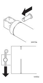
6 Replace cotter pin through hole in pin, bending ends to secure.
