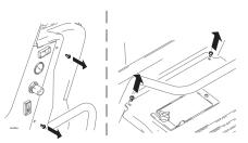
2 Lift cover up and then tilt it back and off sprayer frame.
