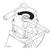
2 Remove 3 screws in side of motor cover. Remove cover.
