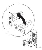
6 Slide pump hose around rollers. Make sure the rollers are horizontally parallel to each other.
