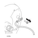
7 Remove 3 screws on right side of cover and remove cover.
