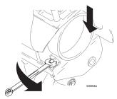
9 Remove single shoulder bolt on other side of motor completely.
