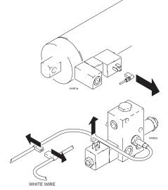
Rotate counter-clockwise to remove sensor from manifold.
