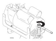
4 Replace end cover. Replace and tighten 3 screws.
