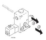
5 Remove Relief Valve from sprayer frame.
