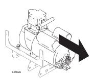
11 Completely remove old shoulder bolts and rubber mounts.
