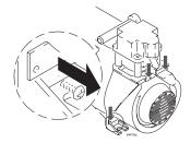
6 Remove bolts and housing from motor.
