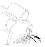
8 Replace reattach green ground wire and grounding nut.
