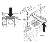
3 Using a screw driver for leverage, lift up on motor support rod on one side of motor and ease it out of the holding bracket far enough to remove old belt. Discard old belt.
