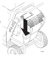
2 Replace and tighten screws.
