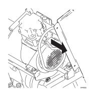
5 Loosen 4 bolts on top of motor housing.
