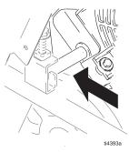
2 Loosen 2 bolts (1 each side) holding down support rod.
