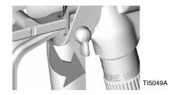
6. Open drain valve. Leave drain valve open.
