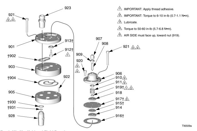
Fig. 9. Mix Manifold and Fluid Regulator
