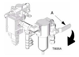
2. Place the ram UP/DOWN lever in the UP position.
