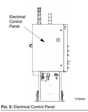
Have a trained electrician connect the electrical control panel (Fig. 5) to a grounded electrical source that has the required service ratings, see **Electrical Requirements** on page 15.
