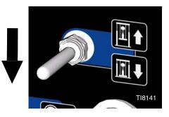
b. Move the ram UP/DOWN lever to the UP position until all air is exhausted from the other side of the ram.
