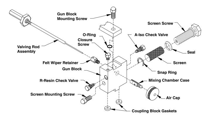
Fig. 2: Centerline Components
