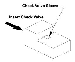
Fig. 24: Sleeve Removal Block
