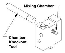
Fig. 22: Mixing Chamber Removal
