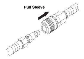
Fig. 5: Air Hose Connection
