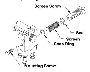
Fig. 17: Filter Screen Assembly
