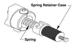
Fig. 20: Retainer Case Removal
