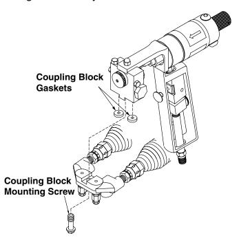
Fig. 3: Coupling Block
