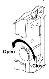
Fig. 7: Air Valve Adjustment
