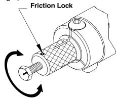
Fig. 6: Valving Rod Adjustment Screw
