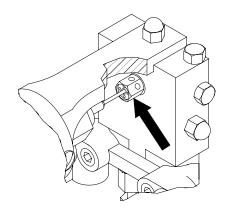
Fig. 8: Felt Wiper
