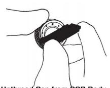
Fig. 27: Unthread Cap from PCD Body
