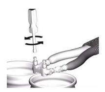
Fig. 21: Open Manual Valves
