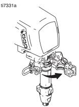
10. Pull out pump pin and place in pin holder.
