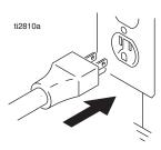
120 Vac: A 12 AWG, 3 wires with grounding prong, 300 ft (90 m) extension cord may be used. 220-240 Vac: You may use a 3-wire, 1.0 mm (12 AWG) (minimum) extension cord up to 90 m long. Long lengths reduce sprayer performance.
