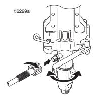
6. Tighten latch and rotate latch lock into locked position.
