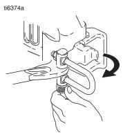
f. Place u-bolt on pump door protrusion.
