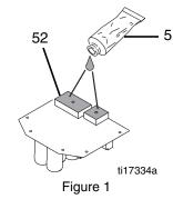
b. For 6 capacitor boards with the powerbar shown in Fig. 2 below, apply a small amount of thermal compound 15U114 or 110009 (5) into both pockets of the Powerbar (69) and scrape across the pocket with the provided scraper so an even layer is remaining in the pocket
