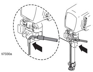
8. Fill pump with Graco TSL until fluid flows onto top of seal.
