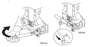
7. Attach drain hose to sprayer.
