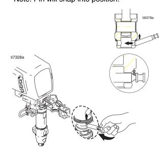
4. Close pump door and rotate latch into position. Do not tighten latch.
