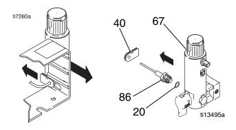
6. Remove grommet (40) from transducer and save for reuse.
