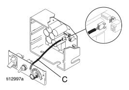
4. Remove four screws (39) and control box (61). Allow control panel (68) to hang down freely.
