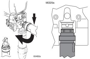
3. Slide pump into connecting rod. Push pump pin until it is fully retained. Note: Pin will snap into position.
