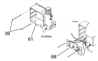
4. Connect potentiometer connector (C) to motor control board.
