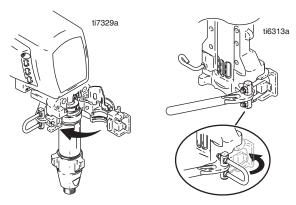
5. Rotate pump to align with paint hose. Connect paint hose and hand tighten to 70 in-lb.
