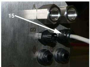
Fig. 19: RoboMix II Strain Relief Fitting
