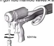
11. Disengage gun piston safety lock.
