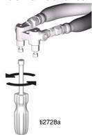
3. Attach gun fluid manifold. Connect gun air line. Open air line valve.
