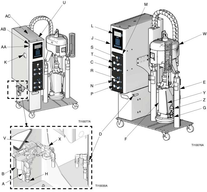
Fig. 1: Component Identification
