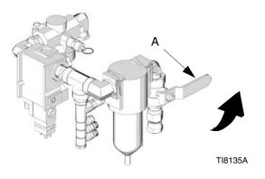
3. Disengage trigger lock.
