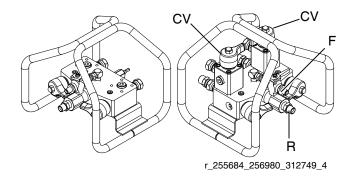
Fig. 4: Remote Mix Manifold Options on Carriage
