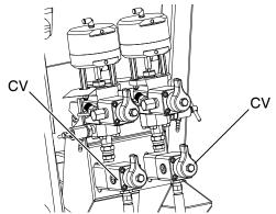
Fig. 3: Machine Outlet Check Valves
