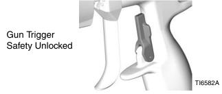
Fig. 4. Trigger Lock
