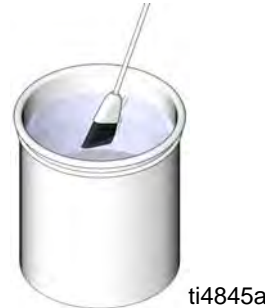
FIG. 14: Use solvent-dipped soft-bristle brush
