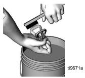
Wipe paint off outside of gun using a soft cloth moistened with water or flushing solvent.
