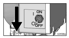
9. Plug power supply cord into a properly grounded electrical outlet.
