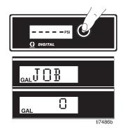
Press and hold display button to reset to zero, or short press button to move to Lifetime Gallons (or Liters x10).
