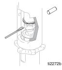
5. Loosen jam nut. Unscrew pump.
