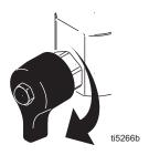
Raise displacement pump above flushing fluid and run sprayer for 15 to 30 seconds to drain fluid. Turn hydraulic valve OFF. Turn engine OFF or turn electric motor OFF and unplug.
