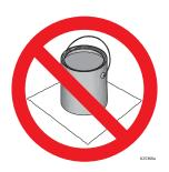
Always ground a metal pail: connect a ground wire to the pail. Clamp one end to the pail and the other end to a true earth ground such as a water pipe.
