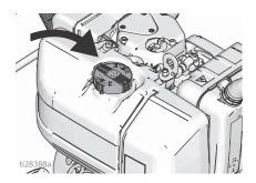
Check hydraulic oil level. Add only Graco Hydraulic Oil, ISO Grade 46, 169236 (5 gallon/18.9 liter) or 207428 (1 gallon/3.8 liter). Hydraulic tank capacity is 1.25 gallon (4.75 liters).
