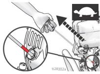
Without releasing the starter rope handle allow the rope to rewind completely.
