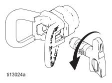
Screw assembly onto gun. Tighten.
