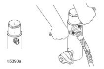
2. Install hose to spray gun and tighten securely.
