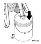
13. Trigger gun again into flushing fluid pail until paint appears.
