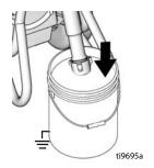
12. Trigger gun again into flushing fluid pail until paint appears.
