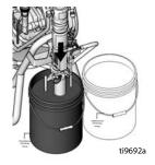
2. Turn prime valve down. Turn pressure control counterclockwise to lowest pressure.
