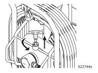
Pull reel handle down and turn clockwise to reel in hose.
