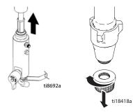
Fill throat packing nut with TSL to prevent premature packing wear. Do this each time you spray.
