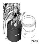
Turn motor switch ON or turn engine ON and start engine. Turn hydraulic pump valve ON. Turn prime valve forward to SPRAY position.
