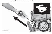
e. After engine starts move throttle lever to MAX (full throttle) position.
