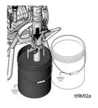
Turn prime valve down to DRAIN position. Turn pressure control counterclockwise to lowest pressure.
