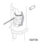
5. Loosen jam nut. Unscrew pump.
