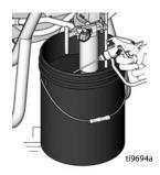
While continuing to trigger gun, turn prime valve down. Then release gun trigger. Allow flushing fluid to circulate until fluid comes out of drain tube clear.
