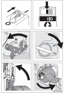
Hold gun against pail. Disengage trigger lock. Turn pressure control up until motor begins to drive pump. Trigger gun until flushing fluid appears.
