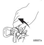
Remove displacement pump from paint and place in flushing fluid. Use water for water-based paint and mineral spirits for oil based paint.
