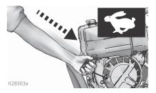
d. Start the engine by pulling the rope using a firm steady pull.
