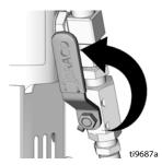
Increase pressure enough to start hydraulic motor stroking and allow fluid to circulate for 15 seconds; turn pressure down, turn prime valve horizontal.
