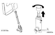
Unscrew and remove inlet strainer.
