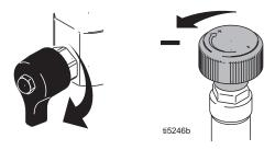
Set hydraulic pump valve OFF.
