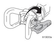
2. Engage trigger lock. Return Switch Tip to original position. Disengage trigger lock and continue spraying.
