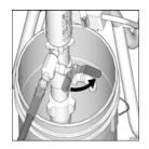
Raise displacement pump above flushing fluid and run sprayer for 15 to 30 seconds to drain fluid. Turn hydraulic valve OFF. Turn engine OFF or turn electric motor OFF and unplug.
