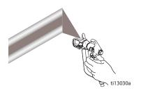
2. Hold gun perpendicular, 10-12 in. (25-30 cm) from surface. Spray back and forth. Overlap by 50%. Trigger gun
