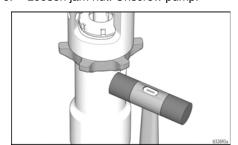
Push retaining ring up; push out pin.
