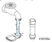
4. Clean cup if not using a liner, and fill with water or appropriate flushing fluid.
