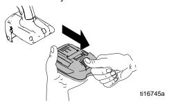
3. Remove pump outlet cap.
