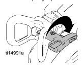
3. Aim sprayer at waste area, disengage trigger lock, and put prime/pressure relief valve DOWN to spray position. Pull trigger to clear clog.
