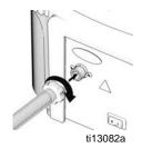
2. Connect air hose from sprayer to inlet fitting of gun.
