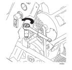
Using a screw driver for leverage, lift up on motor support rod on one side of motor and ease it out of the holding bracket far enough to remove old belt. Discard old belt.
