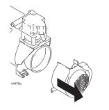
6. Remove bolts and housing from motor.
