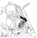
7. Remove 3 screws on right side of cover and remove cover.
