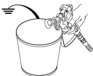
4. Put the suction tube into a grounded metal pail with 1/2 gallon of compatible solvent.
