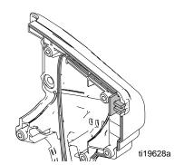
3. Set motor housing into right half of clamshell and loosely install two bolts (42) to motor housing as shown below.
