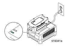
3. When battery becomes fully charged, immediately unplug the charger from the power supply and remove the battery from the charger.
