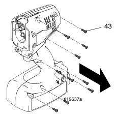
6. Remove trigger lock from assembly.
