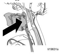
6. Insert trigger lock over trigger with o-ring facing out.
