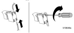
Install trigger over top of wires. Route trigger wires behind trigger.
