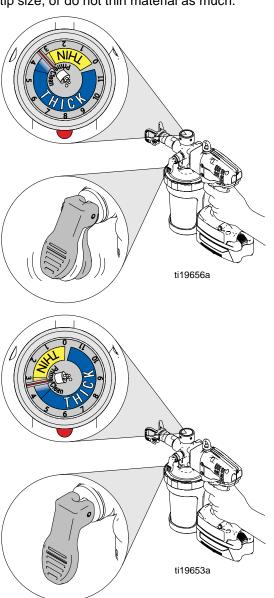
**NOTE:** Thin materials will generally require a low setting and thick materials will generally require a high setting.
