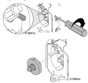
Install pump module to drive module. See Pump Module/Drive Module, page 31.
