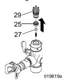
4. Clean as much excess material from inlet cavity as possible.
