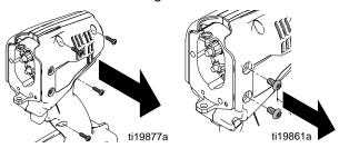
5. Pull the clamshell up and unscrew retaining bolt until gear (48) is no longer retained. Remove gear from drive. Proceed to Installation.
