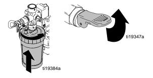
3. Disengage trigger lock, turn sprayer upside-down and trigger for approximately 10 seconds to recircu late material.
