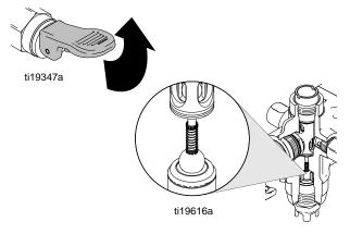
2. Install pressure control knob. Turn knob fully counter-clockwise ("0" setting will line up with red dot). Torque set screws (34) to 40 in-lb (4.5 N•m).
