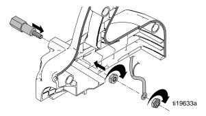
8. Insert static wick into right half of clamshell and install left clamshell to right clamshell.
