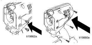
7. Install pump module to drive module. See **Pump Module/Drive Module**, page 31.
