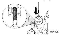
Make sure prime/pressure relief valve is in UP position. Insert ball (27) and assemble inlet fitting (29) using wrench or socket. Tighten to 140 in-lb (15.8 N•m).
