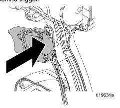
3. Install trigger lock over trigger with o-ring facing out.
