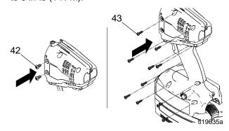
10. Install pump module to drive module. See **Pump Module/Drive Module**, page 31.
