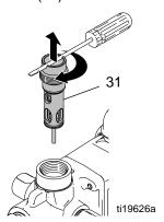
5. Clean as much excess material from outlet valve cavity as possible.
