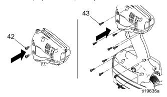
5. Install pump module into drive module. See **Pump Module/Drive Module**, page 31.
