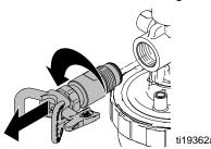
3. Filter should come out of pump housing with valve. If filter remains in housing, remove it by hand or with pliers if necessary.
