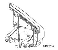
3. Set motor housing into right half of clamshell and loosely install two bolts (42) to motor housing as shown below.
