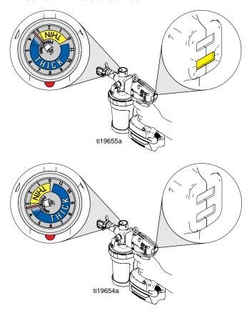
6. If pressure relief valve is vibrating, pressure is set too high. You **MUST** turn down pressure, increase tip size, or do not thin material as much.
