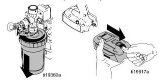
3. Unscrew swivel bolt (22) by pressing down and turning it counter-clockwise. Use tool if needed.
