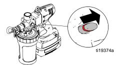
Trigger Unlocked (red ring is visible)
