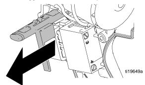
7. Remove trigger switch from clamshell and loosen screws connecting wires to switch.
