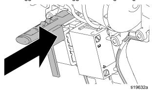
7. Press ground stud into left half of clamshell. Tighten nut onto stud. Install ground terminal to stud and tighten second nut onto stud. Install wire up along handle.
