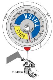
If yellow light is flashing while triggering, pressure is set too high. You MUST turn down pressure until yellow light no longer flashes, increase tip size, or do not thin material as much.
