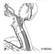
5. Assemble trigger over top of wires. Route trigger wires behind trigger.
