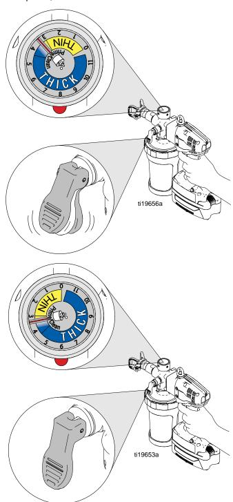
**NOTE:** If not enough pressure can be achieved for an acceptable pattern, reduce tip orifice size and repeat steps. If acceptable pattern is still not achieved, material might need to be thinned or heated (see material manufacturing data sheet for thinning and heating instructions).
