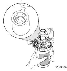
**NOTE:** To purge the maximum amount of air out of the liner, slightly tilt the sprayer so the check valve is the highest point.
