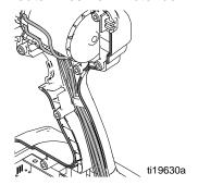
Install trigger over top of wires. Route trigger wires behind trigger.
