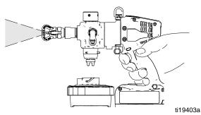
11. Put prime/pressure relief valve UP and pull trigger to finish flushing material.
