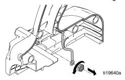
Remove motor, motor housing, switch, control board, indicator lights, trigger lock, and static wick from clamshell.
