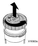
5. Remove material liner and lid from cup and properly dispose. Properly dispose any excess material left in the liner.
