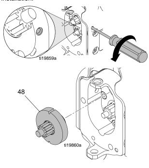
4. Remove four screws holding clamshells together and two bolts connecting drive to clamshell.
