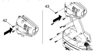
10. Install pump module into drive module. See **Pump Module/Drive Module**, page 31.
