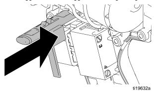
4. Install bolts (42) into motor housing and install screws (43) to connect the clamshell halves. Make sure LED lights and static wick are properly in place. Tighten all four bolts (42) to 50 in-lb (5.6 N•m) and screws (43) to 9 in-lb (1 N•m).
