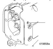
3. Unscrew retaining bolt until gear (48) is no longer retained. Remove gear from drive. Proceed to Installation.
