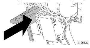
7. Install ground terminal to stud and tighten second nut onto stud. Install wire up along handle.
