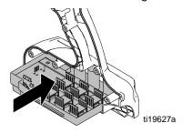
Install two LED lights into designated slot in right half of clamshell. Push wire bundle into slots in clamshell.
