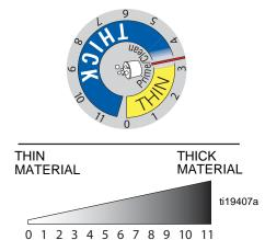
3. Dial in pressure by spraying material on a scrap material.
