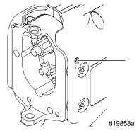
Install new gear into drive housing. Screw retaining bolt into drive housing to retain gear. Torque to 30 in-lb (3.4 N•m).
