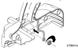
8. Insert static wick into right half of clamshell and install left clamshell to right clamshell.
