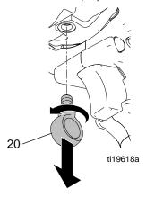
5. Remove pump module (35) from drive module (11).
