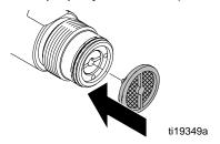
5. Reassemble valve housing to pump.
