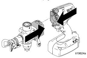
5. Install new gear into drive housing. Pull the clam shell up and screw in retaining bolt to retain gear. Torque to 30 in-lb (3.4 N•m).
