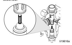
Install pressure control knob. Turn knob fully counter-clockwise until it stops ("0" setting will line up with red dot). Torque set screws (34) to 40 in-lb (4.5 N•m).
