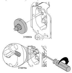
Install two bolts connecting drive to clamshell.
